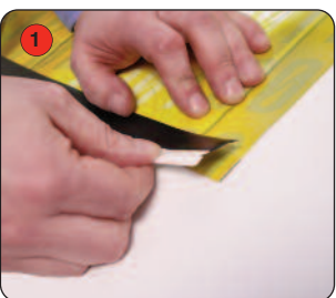
1 Align and adhere the graphic squarely to the slider strip. (attach to front face of graphic)
